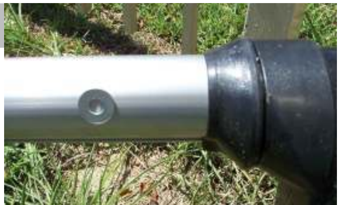
Example of washer and magnet in open position (closed for push-to-open)
